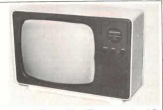
The mighty monitor! The Micron 300 mm (12") green screen monitor must offer just about the best value for money you can get in a computer monitor. Whilst it does feature 10 Hz to 20 MHz bandwidth and high resolution, like many others you see around, it has the unique feature of 'reverse picture' capability. By simply turning up the brightness and turning back the contrast — presto, instant black-on-white!
