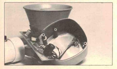
Insides out. The amplifier board mounts inside the rear cover of the Benelec 8-224 horn.
