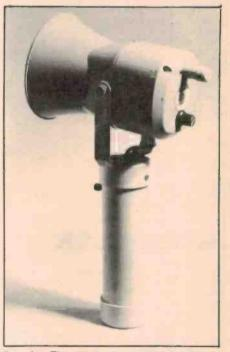
Rear view. The mic plugs into the DIN socket at the top. The volume control is below it. The 'handle' houses the batteries.
